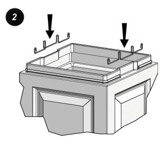
Align the hooks along the recessed areas and slip the brackets over the lip of the bin.
