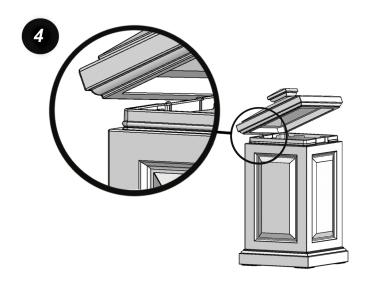
Snap fit lid design for secure fit.
